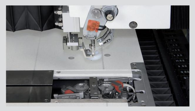
Bobbin thread monitor and needle thread monitor via sensor
