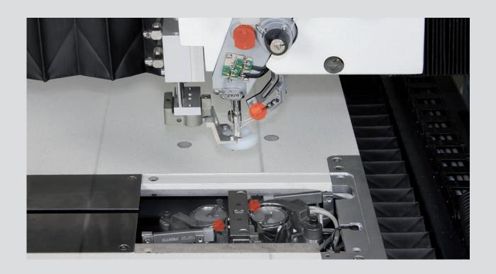
Controlled thread nippers (top and buttom) ensure a reliable seam start
