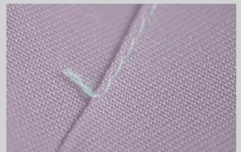
Clean-cut at end of the seam (< 5mm)
