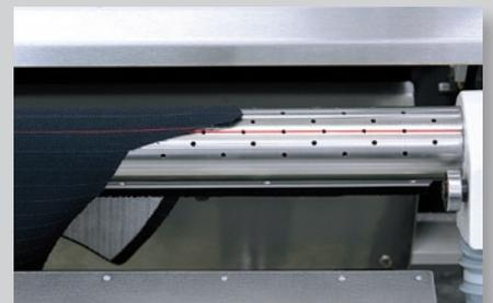
Laser beam for exact placing and positioning of the material
