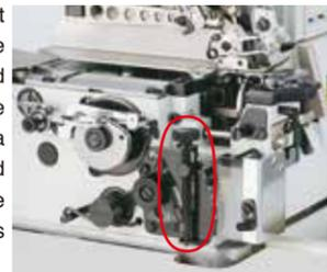
Differential-feed micro-adjustment mechanism
