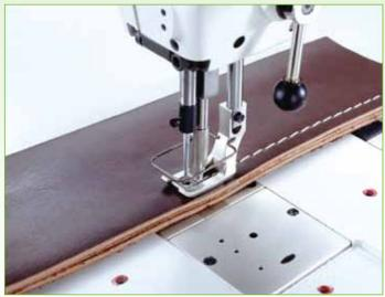
The machine is optimally suited for the sewing of extra-heavy-weight materials such as tents, seat belts, and bag handles.
