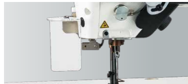
A: Eye guard with an open / close sensor
