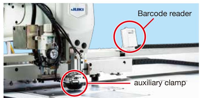
※ The barcode reader reads the barcode on the cassette clamp and automatically selects the corresponding sewing pattern.
