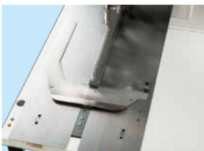
When performing welting of slacks and working pants, the pocket bag presser device clamps the pocket bag for sewing it simultaneously with welting.
