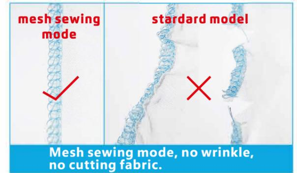
Mesh sewing mode, no wrinkle, no cutting fabric.
